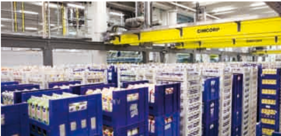
The MultiPick Dual gripper can handle two crate stacks at a time, doubling the handling capacity.
