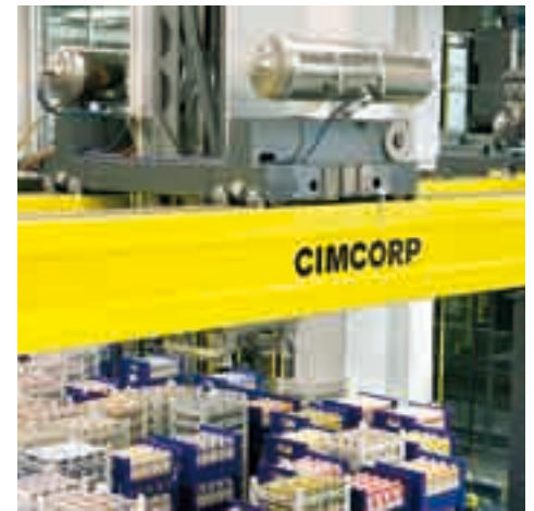
The MultiPick Dual gripper can handle two crate stacks at a time, doubling the handling capacity.
